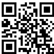
Figure 1. QR code<sup>1</sup>, encoding the text “ABCDEF01”.
