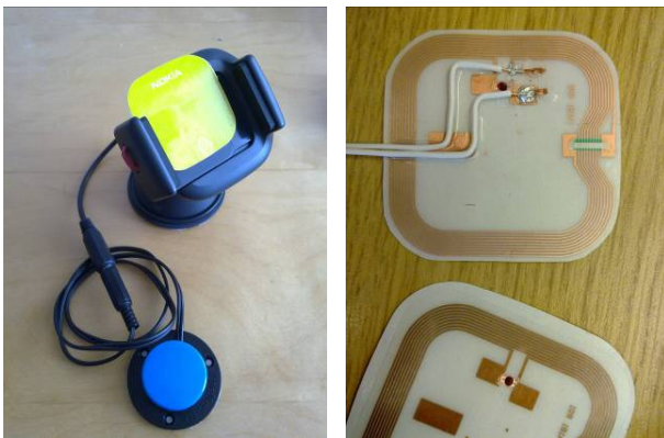
Figure 3. Modified tag attached to mobile phone cradle with connected switch (left). NFC tag with attached cable for switch connection (top right) and original tag (bottom right).
